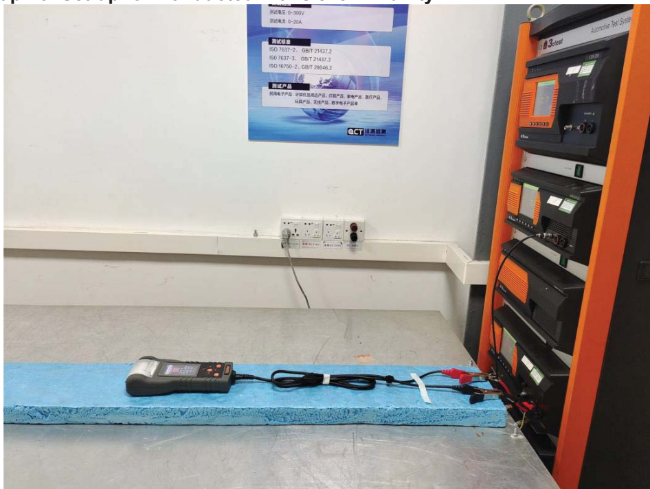
Photograph 3: Set-up for Conducted Transient Immunity
